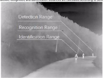
Detection Range: In order to distinguish an object from the background, the object must be covered by 1.5 or more pixels.
